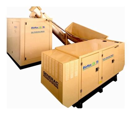
BioMax® units have already demonstrated the ability to successfully gasify wood chips, wood pellets, grass pellets and grass cubes, as well as corn. Gasifiers, such as the CPC BioMax® units, work better if their fuel supply is consistent in character: size, moisture content, energy content etc. Standardized grass pellets and cubes for use in a modular biopower system would eliminate the labor and machinery costs required to chip, sort, dry, and remove tramp materials from green wood.
